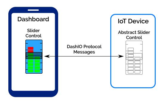
System Messages are also used for purposes other than controls messaging, for example to setup connections and deliver configuration and alarm messages.
