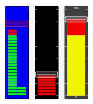
Sliders allow the user to send a numerical values to the IoT device when the user drags the slider to a new position. The slider also includes a single or double bar graph that can be set by the IoT device. The bar graphs can be controlled independently of the slider or can be used to provide feedback to the user from the IoT Device.
