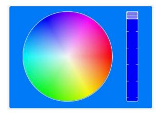
A Color Picker control is used to select a color to send to the IoT device. The Color Picker may be shown as either a spectrum or as a color wheel and brightness slider.
