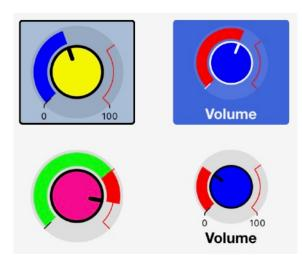
A Knob allow the user to send numerical values to the IoT device when the user drags the knob to a new position. A Knob control contains a user adjustable knob surrounded by a simple dial indicator. The dial can be controlled independently of the knob or can be used to provide feedback to the user from the IoT Device.
