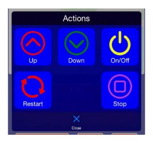
A Button Group control is used to present a popup grid or table of Button controls. The Button Group does not receive messages directly, but presents Button controls that send and receive messages.
