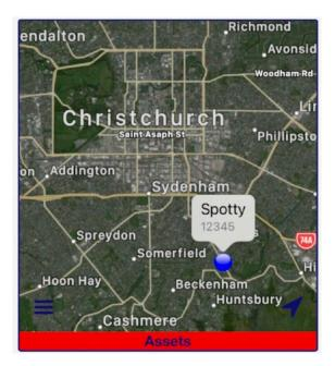
A Map display is used to plot positions on a map. The Map display receives messages from the IoT Device that contain latitude and longitude to mark the position. Additional data, such as speed and altitude may also be included and shown on the Map display.
