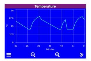
data points and the **Dash** app appends the incoming data to create a data series that can be presented, panned and zoomed by the user. The data may be shown as lines, bars or blocked areas. Each line can be independently added, deleted or changed by the IoT device.
