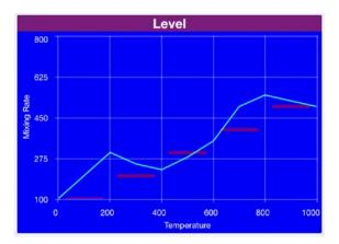
A Chart display is used to present graphical data on the **Dash** app, where the data is a series of vertical (Y) axis data. The data is evenly spaced on the horizontal (X) axis. The IoT device sends a message for each line in the chart. The data may be shown as lines, bars or peak values. Each line can be independently added, deleted or changed by the IoT device.
