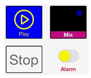
A Button allow the user to send simple action messages, informing the IoT device that the button has been pressed. The button state (**on** or **off** color) is not changed by tapping the button. After the IoT device receives a message containing the action, it sends a message back to the control on the **Dash** app to set the button state.
