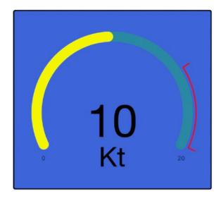
A Dial display is used to present a numerical value in a graphical circular dial. The Dial display receives messages from the IoT device to set the dial position.
