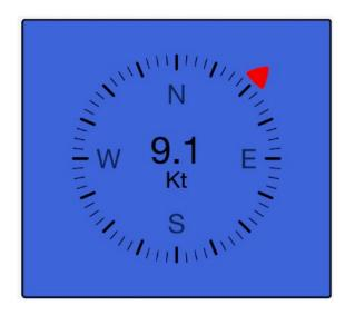
A Direction display is used to graphically present a decimal direction value from 0 to 360 degrees. The Direction display receives messages from the IoT device to set the direction indicator position.
