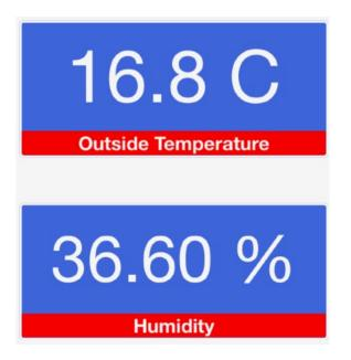
A Text Box control receives simple line text messages from the IoT device to display on the **Dash** app. The text may optionally be plain text, reformatted as a number or, when the text is ISO8601 date/time, it may be formatted to a date/time that is easy to read.
