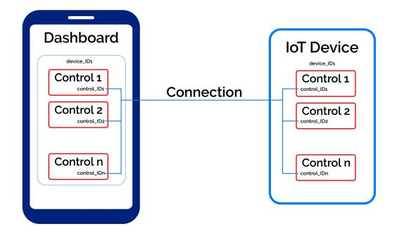
Controls for a device are displayed on the Dash IoT Dashboard on a graphical feature called a **Device View**. There may be one or more Device Views for an IoT Device. The device view contains a "theme" of layout features and colors that are common to all controls displayed on the Device View.
