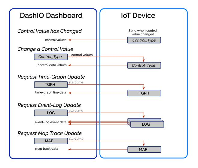
The Time-Graph (TGRPH), Event-Log (LOG) and Map (MAP) *Control\_Type* request messages from the Dash IoT Dashboard are used to request updated Time-Graph, Event-Log and Map information respectively. These request messages include a **start time**, which indicates to the IoT device that the Dash IoT Dashboard only requires information from AFTER the start time.
